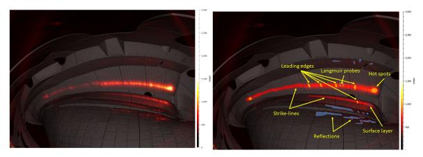
There are safety strategies to stop the experiments when critical areas get too hot (Fast Interlock System). The objective of the current proposal is to estimate when this will happen and cool down the system before it has to be stopped. It will rely on previous works carried out at UPC:
